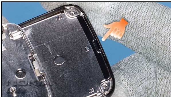
5. Mind the correct positioning of the metal latch of the C-COVER ASSEMBLY when reassembling the UI-COVER.
